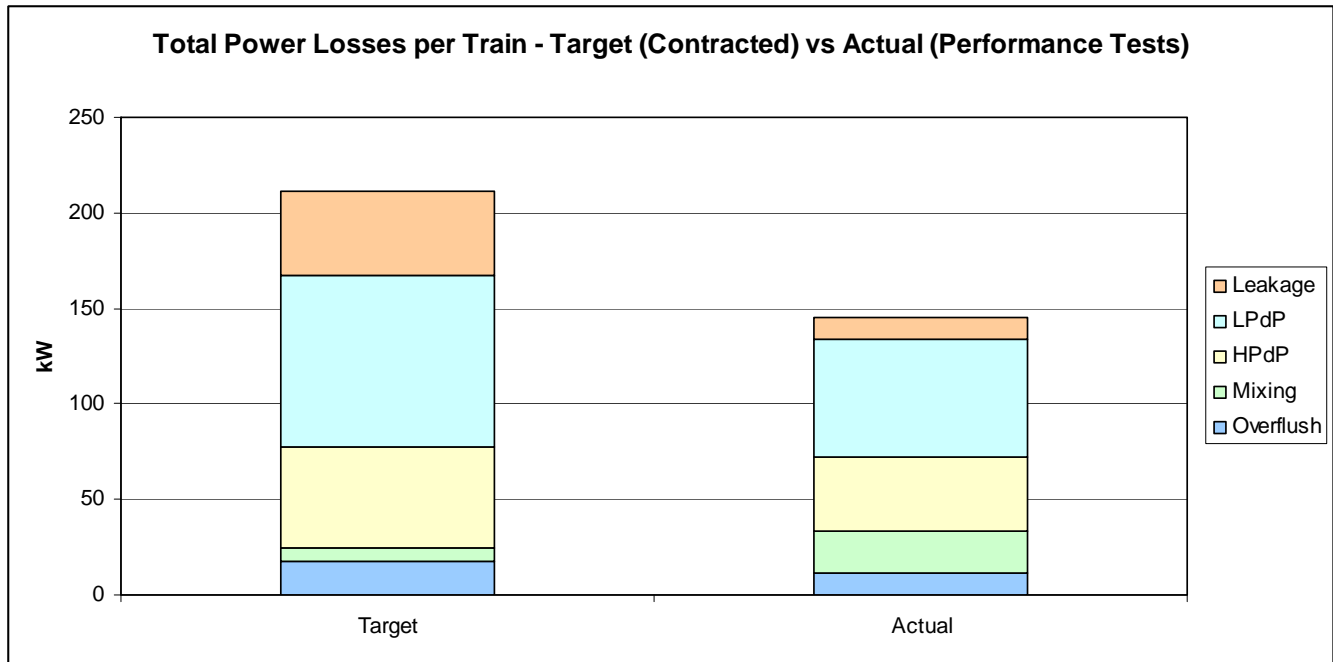
Figure 5: Target (contracted) and actual power losses of the DWEER ERD in Sydney
