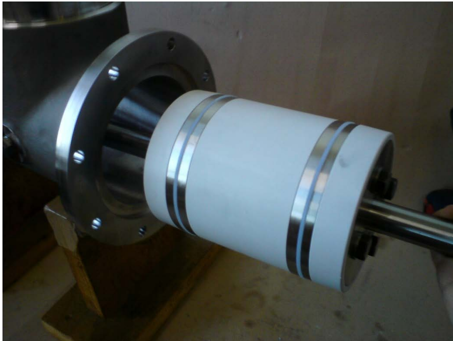
Figure 4: Double LinX Piston seal design
